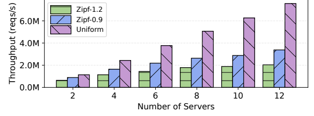
Figure 2: Peak throughput of an HTTP server pool with an existing L4 load balancer, Load-aware Weighted Round Robin (LWRR), under a p99 latency SLO of 100 \mu s. Skewed workloads (Zipfian [43]) across 720 long-lived connections limit server scalability, as existing L4 LBs cannot dynamically alleviate bottleneck servers. Setup details are in §8.
